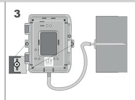
For wall fixing, mount the LEV Monitor in a visible location, insert and screw the spigot into the duct, then connect the monitor and probe using the hose provided.
