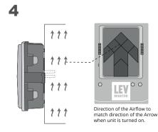
Place the LEV Monitor spigots into the duct with the Arrow pointing in the direction of the Airflow.
