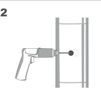
edges are de-burred to avoid tearing the seals.
